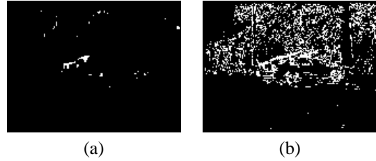
Figure 2. (a)The result of conventional background subtraction. (b) The result of Index of Disparity algorithm processing.
