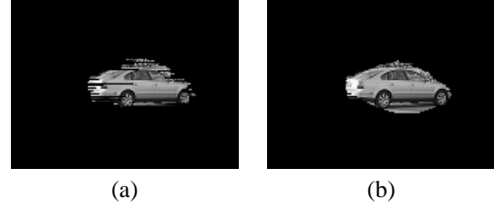
Figure 5. (a)The result of edge completion and filling when no prior knowledge about the geometry is used (b) The result when prior knowledge is included.
