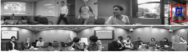
Figure 1. Example panoramic views of two meeting rooms for person detection. In the upper image, the blue box is one of the hand-labeled ground truth heads. The red box is the expanded box that includes shoulder for detector training.
